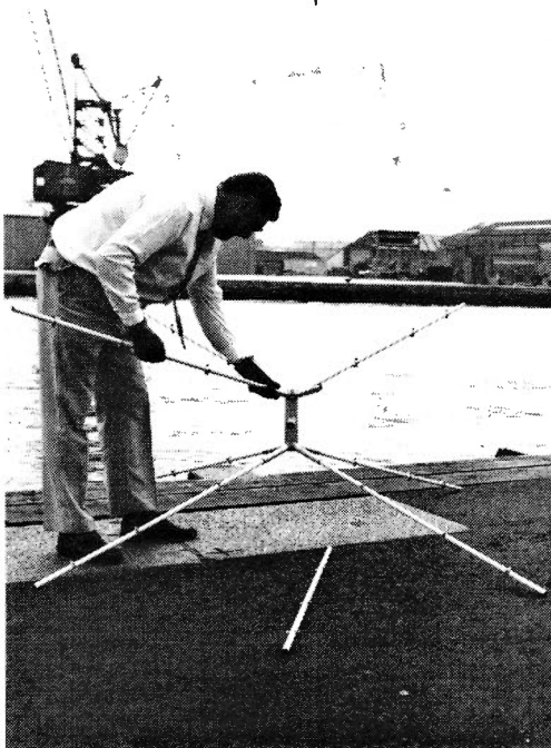
Fig. 2: A demonstration assembly of the Nelson antenna on the Quay at Poole. The sturdy glass fibre spreaders fit into the 'spider', with the loop element holders being spaced out along each spreader. The relatively small size of the three band v.h.f. cubical-quad can be gauged, when it's compared to Tex Swann G1TEX, who bumps his head at 1.9m!
